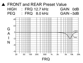
If you want to change the characteristics, follow the procedure below to adjust the frequency and gain for the high-shelving equalizer (HIGH) and parametric equalizer (PEQ). For the more detailed characteristics in different settings, see "CINEMA-EQ Frequency Characteristics" on page 82.
