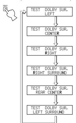
Press **TEST** on the remote control so "TEST DOLBY SUR." appears on the video monitor and front panel display.
