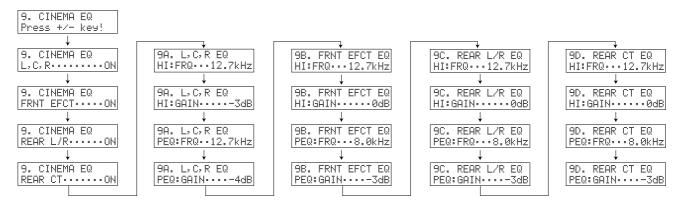
• Each time you press ∇(or **NEXT** ), the parameter changes on the front panel display as shown above. Press the cursor △ to go in the reverse order.
