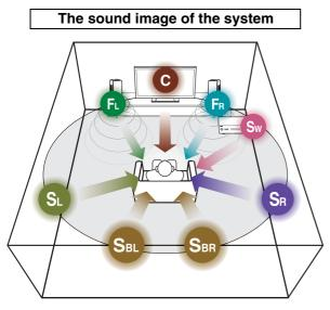
The system creates the virtual 7.1 channel surround sound with the subwoofer integrated receiver and the speaker.
