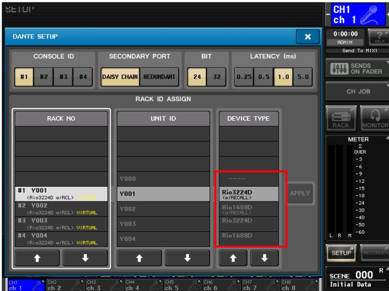
3. In the **DEVICE TYPE** list, set the **DEVICE TYPE** for the I/O rack that you want recalled from the currently selected CL series to an I/O rack indicated by “(w/RECALL)”.
