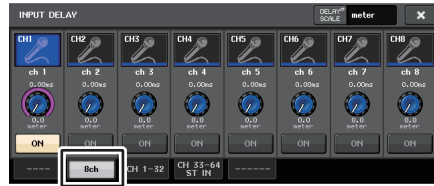
Ventana emergente INPUT DELAY
