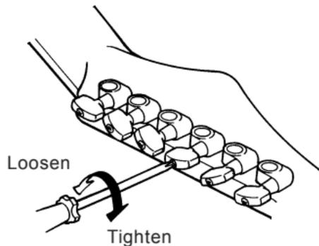
Clockwise screw rotation tightens the machine. The tuning machines should be adjusted to the extent that they are firm, but can turn smoothly. This adjustment is normally unnecessary, and excessive tightening can lead to premature tuning machine wear.
