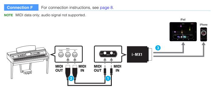
Please make sure that i-MX1 MIDI OUT terminal is connected to the MIDI IN terminal of the instrument, and the i-MX1 MIDI IN terminal to the MIDI OUT terminal of the instrument.
