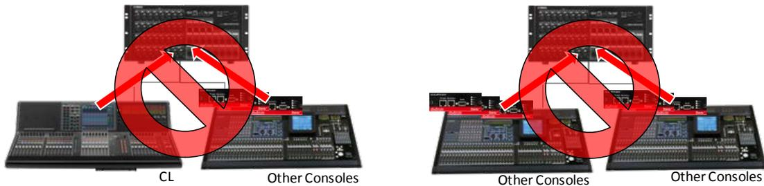
It is only when the R series (in NATIVE mode) is controlled from the CL series that the same I/O rack can be controlled from multiple consoles (in this case, also the Gain Compensation function can be used). However, even on the same network, the HA of a different I/O rack can be controlled from other consoles.
