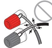
– Do not let the bare wires of the speaker cable come into contact with the unit's metal parts (rear panel and screws).
