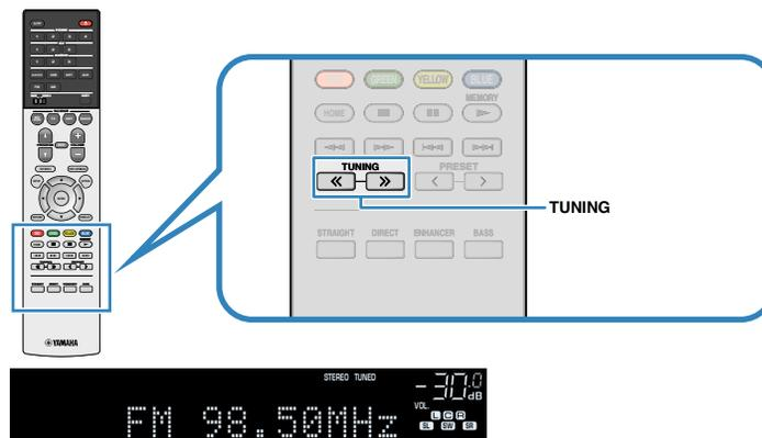
On the front display, “TUNED” lights up when the unit is receiving an FM/AM radio station signal.
