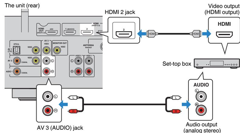
**1** Press HDMI2 to select “HDMI2” (video input jack to be used) as the input source.
