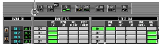
Switch direct out on/off for each channel.
