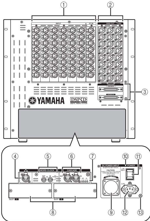
**① INPUT jacks 1–48 / ST IN (stereo input) jacks 1–4**
