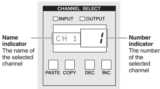
The number shown in the number indicator is as follows. If a channel is paired, the decimal point for the lowest place will light. For a FX RTN channel, the decimal point for the highest place will light.
