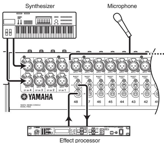
INPUT jacks 1–48 are used mainly to connect microphones or monaural line-level devices. ST IN jacks 1–4 are used mainly to connect stereo line-level devices. Input signal sensitivity, pad on/off, and phantom power (+48V) on/off are controlled from the top panel AD IN section (➔ p.44).
