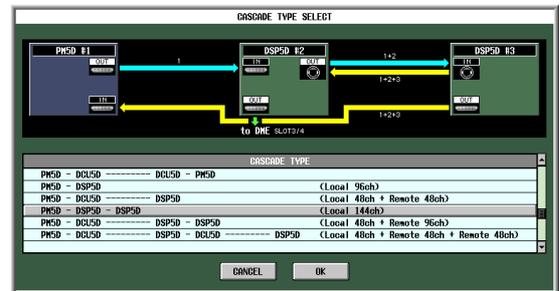
This system cascade-connects two DSP5D units to the PM5D, expanding the number of input channels to 144 monaural input channels.
