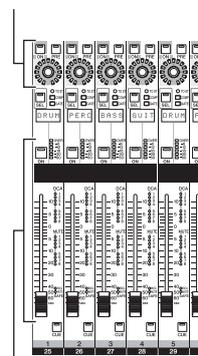
Control the channel input level and on/off status
