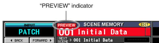
While in PREVIEW mode, operating the knobs, encoders, and other controls (except for the TALK-BACK section, CUE/MONITOR section, and the AD IN section of the PM5D model) will not affect the audio signal processing.
