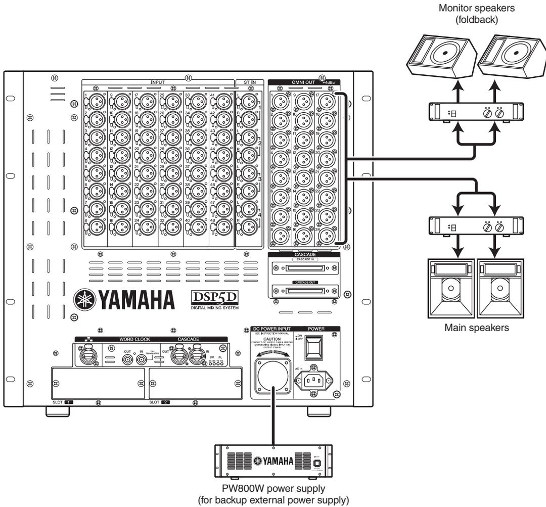
With the default settings, the signals of MIX channels 1–22 are output from OMNI OUT jacks 1–22, and the signals of the STEREO A channel are output from OMNI OUT jacks 23–24. The desired output signal can be patched to each jack; the signals of MIX channels 1–24, MATRIX channels 1–8, STEREO A/B channels, or cue signals can be output from OMNI OUT jacks 1–24.
