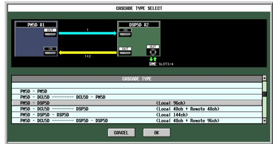
This system cascade-connects one DSP5D unit to the PM5D, expanding the number of input channels to 96 monaural input channels.
