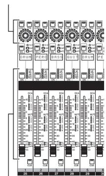
Control the send level and on/off status of the signal sent from the channel to the MIX buses
