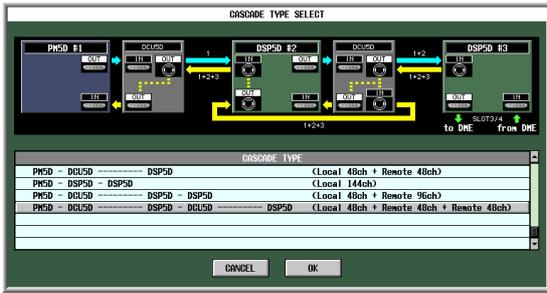
This system cascade-connects two DCU5D units and two DSP5D units to the PM5D, adding two sets of 48 remotely located monaural inputs.
