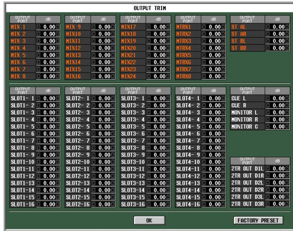
To adjust the gain, click the  $\leftarrow$  /  $\rightarrow$  buttons located at the left and right of each box to specify the gain of each output port in 0.01 dB units. If you want to reset all output ports to 0.00 dB, click the FACTORY PRESET button. Click the OK button to apply the settings.
