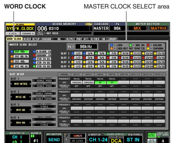
In this screen you can select the master clock, and check the input signal synchronization status for each slot or jack.
