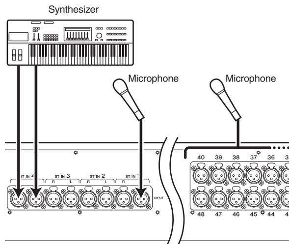
INPUT jacks 1–48 and ST IN jacks 1–4 can both be used to connect microphones or line-level devices. Input signal sensitivity and phantom power (+48V) on/off are controlled from within the display (➔ p.44). However, all phantom power can be switched on/off as a whole by the rear panel [+48V MASTER] switch.
