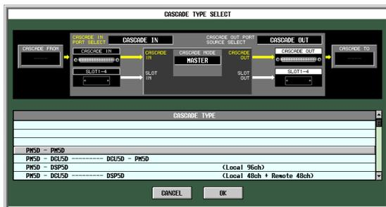
This system directly cascade-connects PM5D units. A maximum of four PM5D units can be connected. Use 12-17 to specify the details of the cascade connection.
