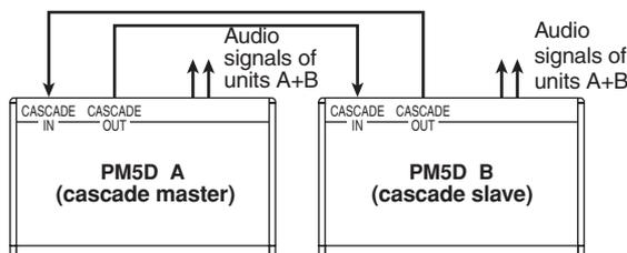
If you want operations such as scene store/recall and cue/solo to be linked between the two PM5D units, specify one unit as the cascade master and the other as the cascade slave. (This setting is made in the SYS/W.CLOCK function MIXER SETUP screen.) The PM5D assigned as the cascade master will output control signals (operational signals) via its CASCADE IN connector, and the PM5D assigned as the cascade slave will receive these signals via its CASCADE OUT connector.
