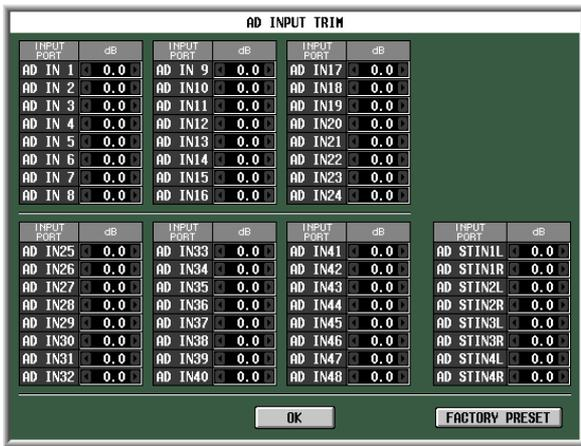
To adjust the gain, click the  $\leftarrow$  /  $\rightarrow$  buttons located at the left and right of each box to specify the gain of each input port in 0.1 dB units. If you want to restore all input ports to their factory settings, click the FACTORY PRESET button. Click the OK button to apply the settings.
