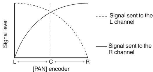
In this case, MIX TO STEREO PAN will operate as a conventional PAN control, and no signal will be sent to the CENTER channel.
