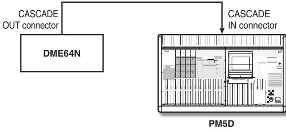
**4 Uni-directional connection using the CASCADE IN/OUT connectors — 2 (DME64N only)**
