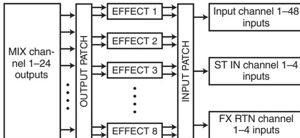
Alternatively, you can insert an internal effect into a channel by assigning the input/output of the internal effect to the insert-out/insert-in of the desired channel.
