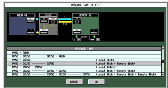
This system cascade-connects one DCU5D and one DSP5D to the PM5D, adding 48 remotely located monaural inputs.
