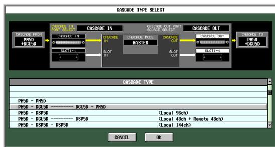
This system cascade-connects two DCU5D units between the PM5D units in order to extend the dis-
