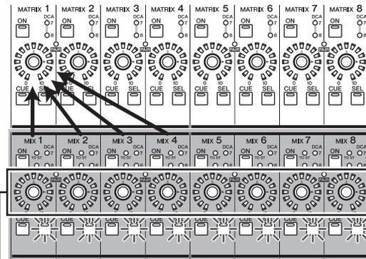
Use the encoders of the MIX section to adjust the send levels
