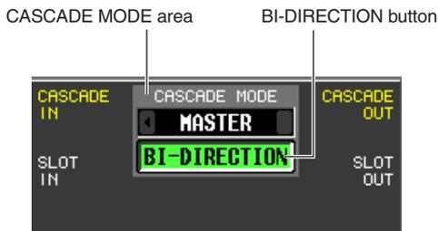
When multiple PM5D units are cascaded, the settings of the CASCADE MODE area specify whether the unit will operate as a cascade master (when "MASTER" is selected) or as a cascade slave (when "SLAVE" is selected).
