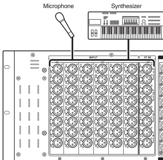
INPUT jacks 1–48 and ST IN jacks 1–4 will accommodate connections ranging from microphones to line level devices. Each connector is provided with phantom power (+48V), and the input signal sensitivity and phantom power on/off can be operated from the display as on the PM5D-RH (➔ p.44). The +48V master switch is turned on/off in the SYS/W.CLOCK function MIXER SETUP screen (➔ p.221).
