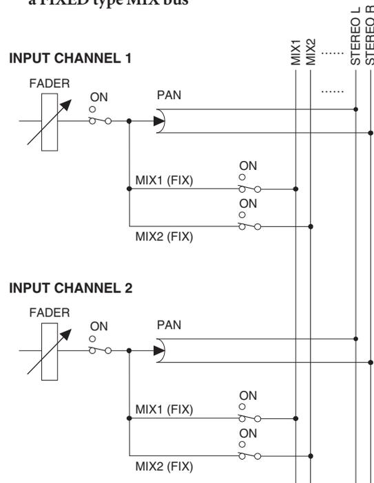
If the send-destination MIX bus is set to FIXED mode, the MIX encoders have no effect; the signal can only be switched on/off by the MIX [ON] key.
