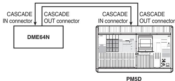
**3 Uni-directional connection using the CASCADE IN/OUT connectors — 1 (DME64N only)**
