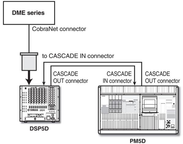
**Procedure for connecting the DSP5D and DME series**
