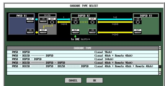
This system cascade-connects one DCU5D and two DSP5D units to the PM5D, adding 96 remotely located monaural inputs.
