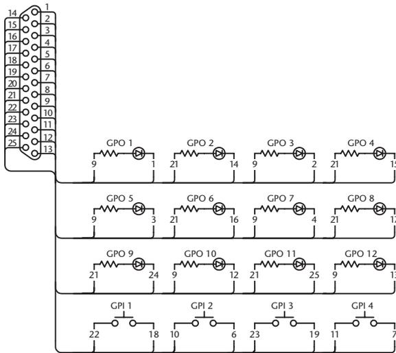
This circuit uses four switches (GPI 1–GPI 4) to switch the GPI IN ports between active and inactive. If the polarity of a GPI OUT port is set to Low Active, and you operate the PM5D to make the GPI OUT port Active, the corresponding LED in the above circuit (GPO 1–GPO 12) will light. (If the polarity of the GPI OUT port is High Active, the LED will go dark.)
