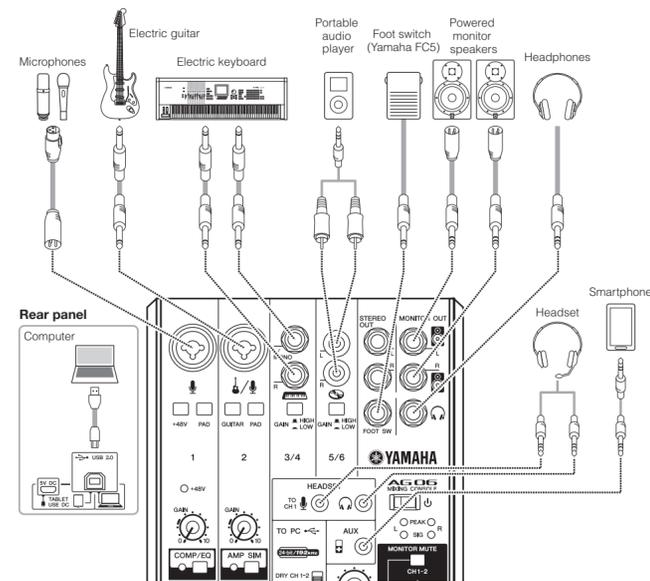
**NOTE** If you are using condenser microphones, turn on ( ) the [+48V] phantom power switch.
