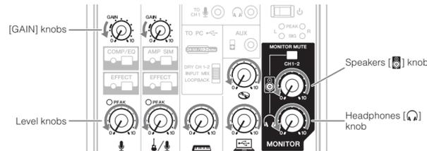
**4 Make sure that the volume of a powered speakers is set to minimum.**
