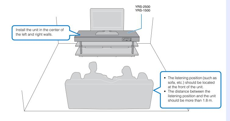
This unit creates surround effects by reflecting sound beams off the walls of your listening room. The arrows in the diagrams on the right indicate the images of paths of 5-channel sound beams. To achieve desired surround sound effects, install this unit where there are no objects such as furniture obstructing the path of sound beams.
