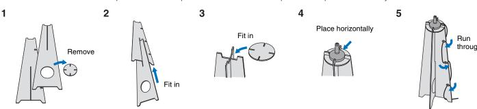
Use the supplied cardboard microphone stand to place the IntelliBeam microphone at the same height as your ears would be when vou are seated
