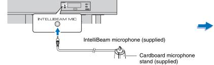
AUTO SETUP (PREPARATION & CHECK) Please place the MIC at least .8m/6ft away from Sound Projector. The MIC should be set lat ear level when seated. asurement takes about 3min After [ENTER] is pressed. ENTER]:Start [RETURN]:Cance
