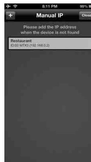
Normally, MTX processors are automatically detected and displayed on the Select Device list. However, in rare cases auto-detection may not be possible with certain Wi-Fi device specifications. In such cases, use the Manual IP function to instead manually add the MTX processor's IP address. Once the IP address is added into the Manual IP list, that MTX processor becomes available on the Select Device list.
