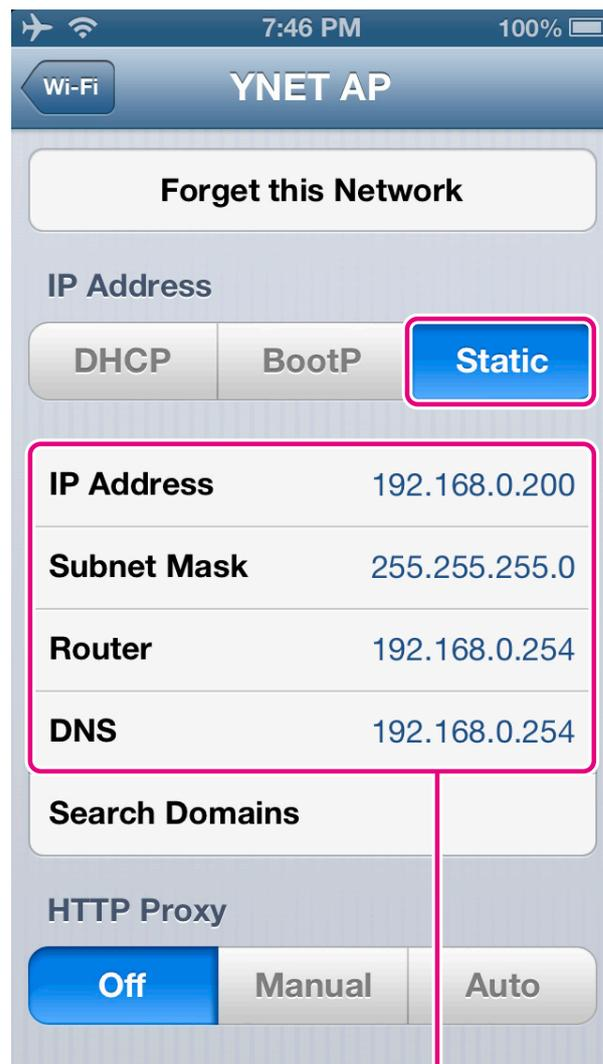
1. IP Address: For the first three numbers, use those from the MTX processor's IP address. Set a different value for the fourth number.
