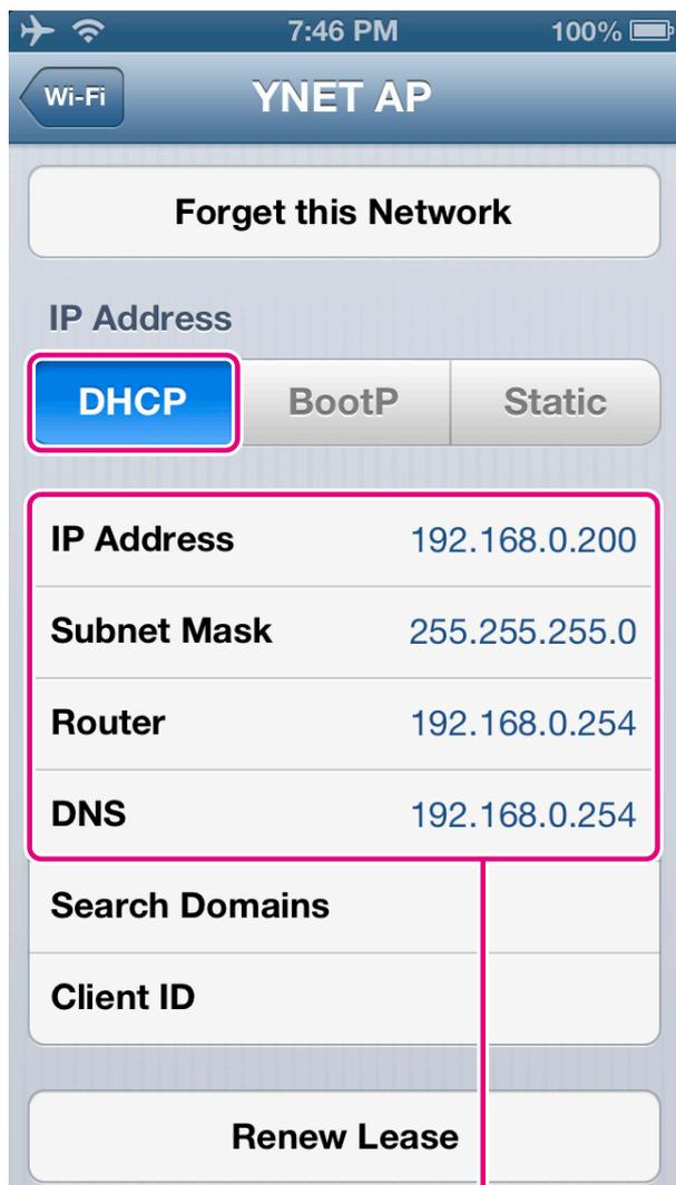
1. Verify that settings have been made for IP Address, Subnet Mask, Router, and DNS.
