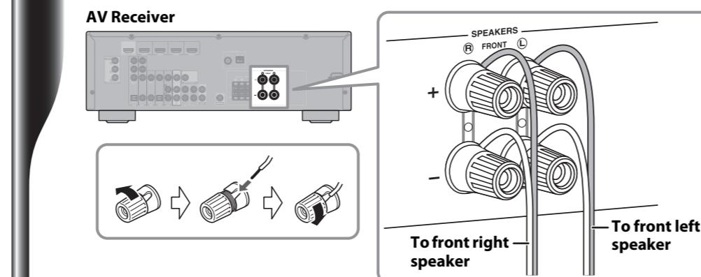
Connect the front speaker (G) cables to the AV Receiver. Make sure you connect the speakers with the correct polarity—positive (+) terminals to positive (+) terminals, and negative (-) terminals to negative (-) terminals.
