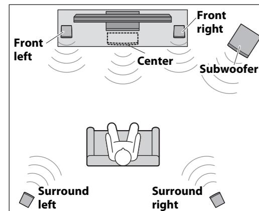
The four front and surround speakers are identical, so it doesn't matter which one you use in each position.
