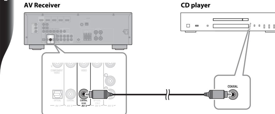
Use an audio pin cable (not included) to connect your CD player to the AV Receiver's AV 3 COAXIAL(CD) jacks, as shown.
