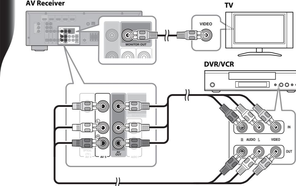
Use a video pin cable (not included) to connect the AV Receiver's MONITOR OUT jack to a composite video input on your TV, as shown.
