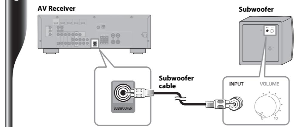
Use the included subwoofer cable (J) to connect the Subwoofer's INPUT jack to the AV Receiver's SUBWOOFER jack.
