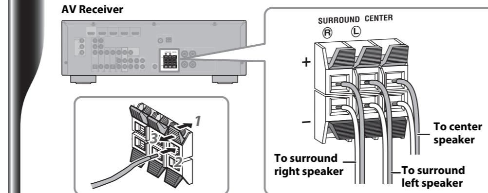
Connect the center speaker (H) and surround speaker (G) cables to the AV Receiver. Make sure you connect the speakers with the correct polarity—positive (+) terminals to positive (+) terminals, and negative (-) terminals to negative (-) terminals.
