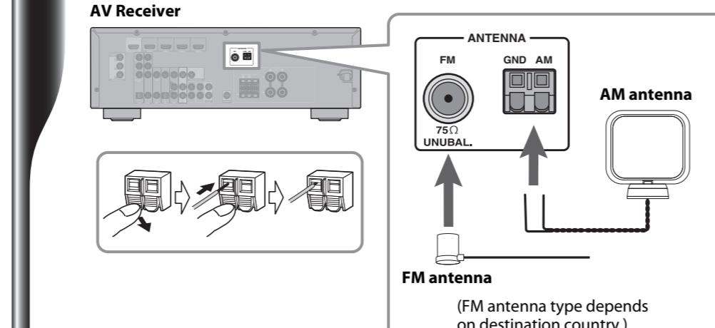
Connect the AM loop antenna (D) and indoor FM antenna (E) to the AV Receiver, as shown. See the owner's manuals for more information about connecting antennas.
