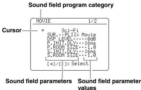
**3 Press one of the sound field program selector buttons (**25**) repeatedly to select the desired sound field program you want to adjust.**
