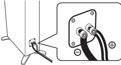
Be sure to connect the “+” (red) and “-” (black) properly. Cables are colored or shaped differently, perhaps with a stripe, groove or ridge. Connect the striped (grooved, etc.) cable to the “+” (red) terminals of this unit and your speaker. Connect the plain cable to the “-” (black) terminals.
