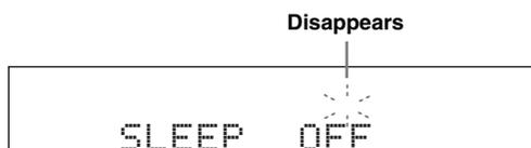
The SLEEP indicator turns off, and “SLEEP OFF” disappears from the front panel display after a few seconds.
