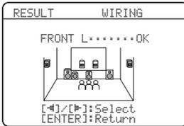
**11** Press **Ⓞ** **</>** repeatedly to toggle between the setup result displays.
