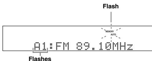
When automatic preset tuning is completed, the MEMORY indicator disappears.
