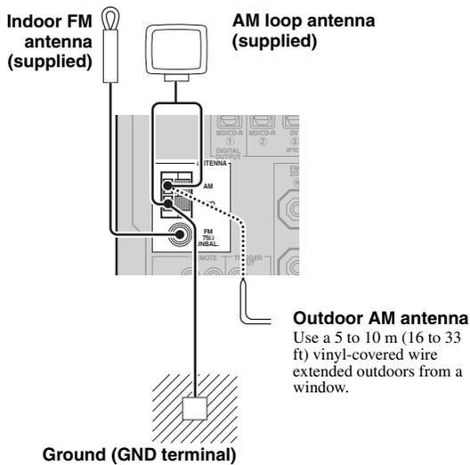
For maximum safety and minimum interference, connect the antenna GND terminal to a good earth ground. A good earth ground is a metal stake driven into moist earth.
