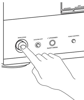
This unit is set to the standby mode and consumes a small amount of power in order to receive infrared signals from the remote control. To turn on this unit from the standby mode, press the desired **Ⓢ SCENE** buttons (or **④ SCENE**) or **Ⓚ MAIN ZONE ON/OFF** (or **Ⓟ POWER**). See page 29 for details.
