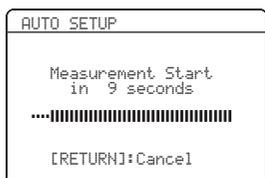
Loud test tones are output from each speaker during the auto setup procedure. Once all items are set, the “RESULT” display appears in the OSD.
