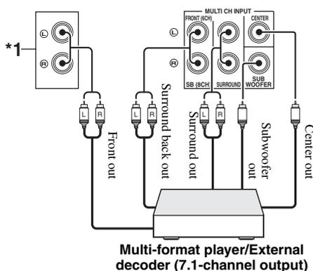
\*1 The analog audio input jacks assigned as "FRONT" in "MULTI CH" (see page 87).
