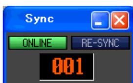
Synchronization between the PM5D itself and PM5D Editor can be switched on/off in this window. This has the same function as the [Synchronization] menu. Click the ONLINE button to switch to off-line, or click the OFFLINE button to switch to on-line. If you click the RE-SYNC button, the Synchronization dialog box will appear (→ p.3). The current scene number is also displayed in this window.
