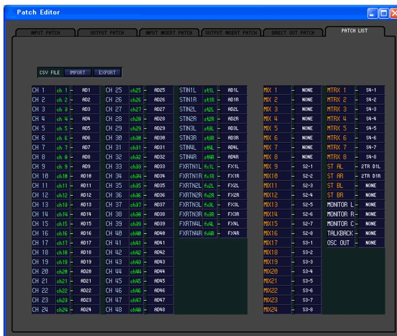
Here you can view and edit the input patch and output patch settings. Input patch, output patch, and channel name data that was written to a CSV file by the PM5D itself can also be loaded into this page. Conversely, the settings in this page can be written to a CSV file that can be loaded into the PM5D.
