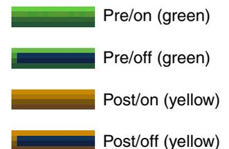
The bar graph display will change according to the send position (pre/post) and on/off status of the signal sent from the input channel to the MIX buses.
