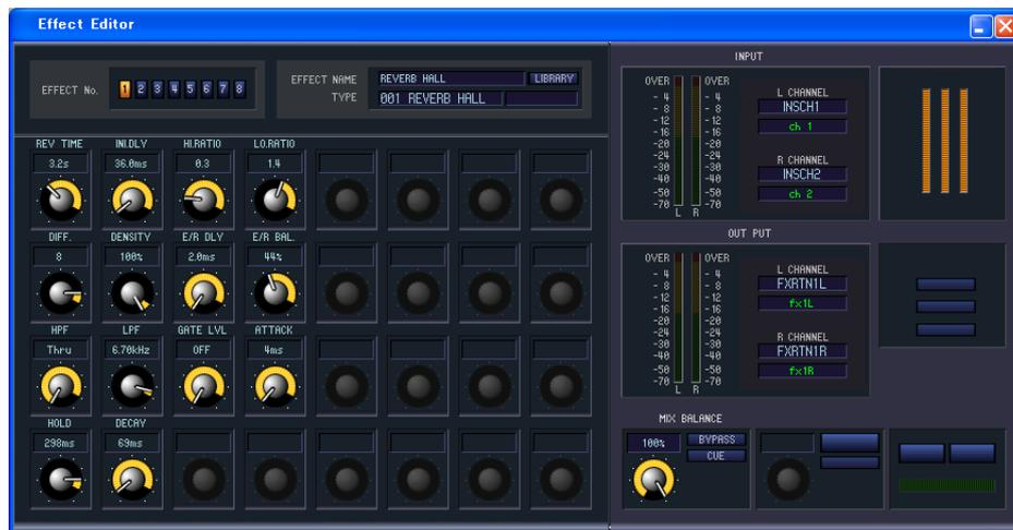
Here you can select the effect type for internal effects 1–8, edit the parameters, and specify the input/output patching.
