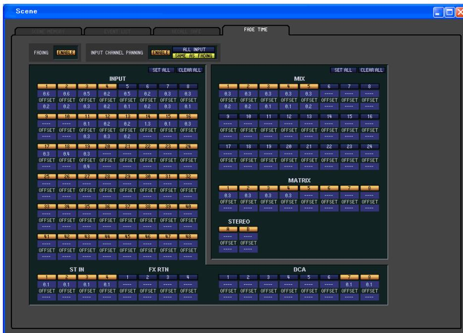
Here you can make settings for the Fade function that adjusts the time over which fader and pan will reach their new values when a scene is recalled. The settings of the Fade function are independent for each scene.
