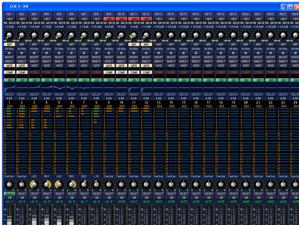
This window displays the mix parameters of input channels 1–24 or 25–48. The window shows either the channel 1–24 layer or the channel 25–48 layer. To open the other layer’s window, choose the [Windows] menu command [INPUT CH] and choose “CH1-24” or “CH25-48.”
