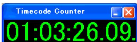
This window displays the time code (LTC, MTC) that the PM5D itself is receiving or generating, in units of hours/minutes/seconds/frames. This is the same time code as displayed in the PM5D's fixed display screen and in the EVENT LIST screen.
