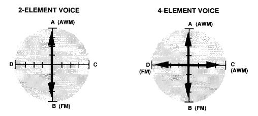
When level vector control is selected, moving the control towards one element (A, B, C or D) increases the level of that element while decreasing the level of the others proportionally. The [VECTOR CONTROL] works in a similar way when detune vector control is selected — moving the control towards one element increases the pitch of that element while decreasing the pitch of the others.
