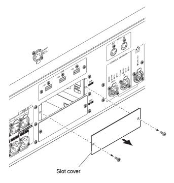
**3.** Align both edges of the card with the guide rails inside the slot, and then insert the card into the slot.
