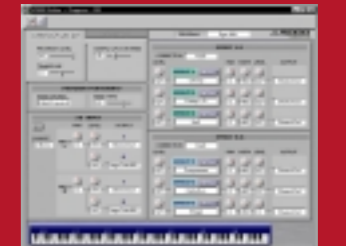
The Program Edit Window lets you quickly edit the parameters related to the A5000/A4000 Program setup, such as effects setup, MIDI channel assignment and Program LFO.
