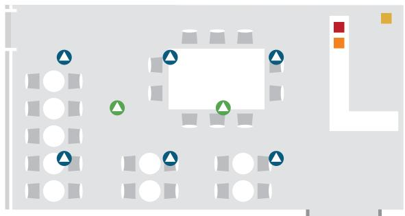
With VXC2F speakers and a mixer amplifier MA2030a, it is possible to create a streamlined, high-performance system that allows microphone use while background music is being played. Add a power amplifier PA2030a and a ceiling subwoofer VXC8S to create enriched ambient.
