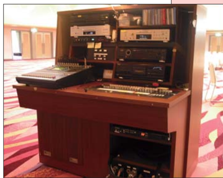
Rack with 01V96 can be moved to any location as far as Ethernet connector is available.
